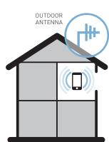
Install **Outdoor Antenna** where the mobile device receives this signal.
